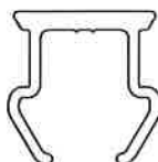
MGS116 POCKET FILLER SINGLE GLAZED (PUSH IN) 0.243 kg/m
