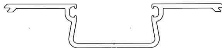
MGS164 POCKET PLATE DOUBLE GLAZED 0.769 kg/m
